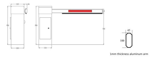
Dimensions of barrier housing & boom arm (mm)
